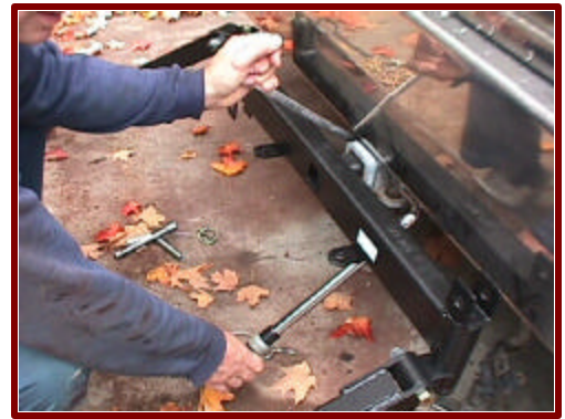
Setting the torque specifications for the coupler/receiver bolt on the coach (above) and the mounting bolts on the towed vehicle (below)
