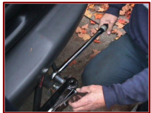
Setting the torque specifications for the coupler/receiver bolt on the coach (above) and the mounting bolts on the towed vehicle (below)
