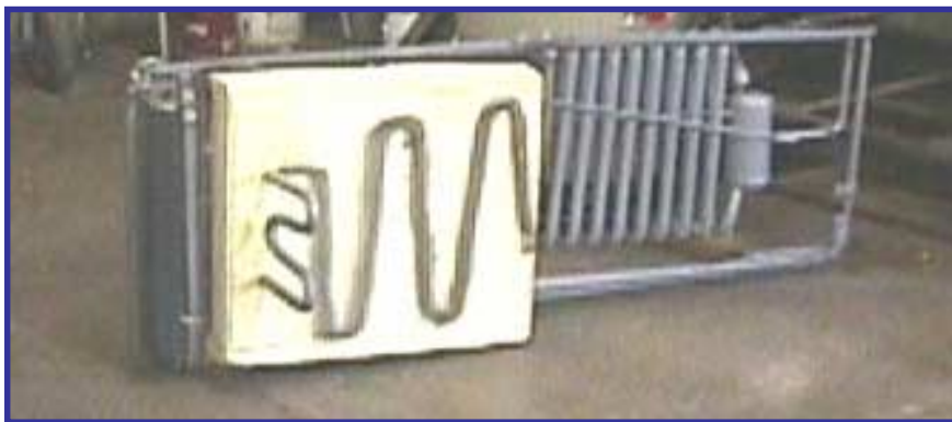
The new evaporator is encased in polyurethane foam
