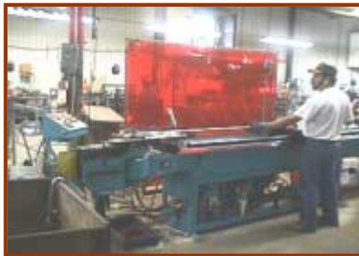
A tube bending machine creates precise duplicates of the evaporator from straight steel pipe.
