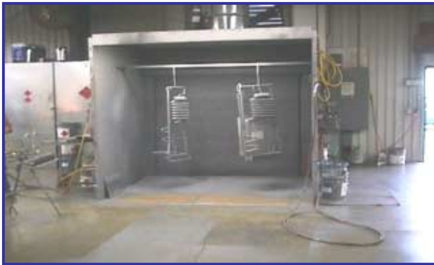
Rebuilt cooling units in the paint booth
