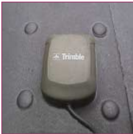
GPS antenna by Trimble. It is mounted between the 3/16" roof rivets
