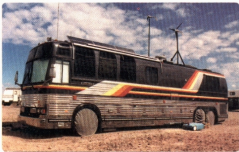
The authors installed wind turbines and solar collectors on their coach's roof to provide them with the power they need to live without hookups (opposite, above).
